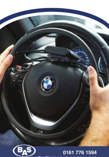
The BAS Ring Accelerator transfers acceleration from the foot pedal to a specially designed ring fitted above (Over Ring) or below (Under Ring) the steering wheel. The linear push motion towards the steering wheel of the Over Ring Accelerator and the pull motion towards the
