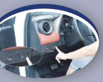
All hatch openers come with a dash mounted switch and a rear mounted boot switch, regardless of make/model of vehicle.
