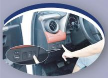
All hatch openers come with a dash mounted switch and a rear mounted boot switch, regardless of make/model of vehicle.
