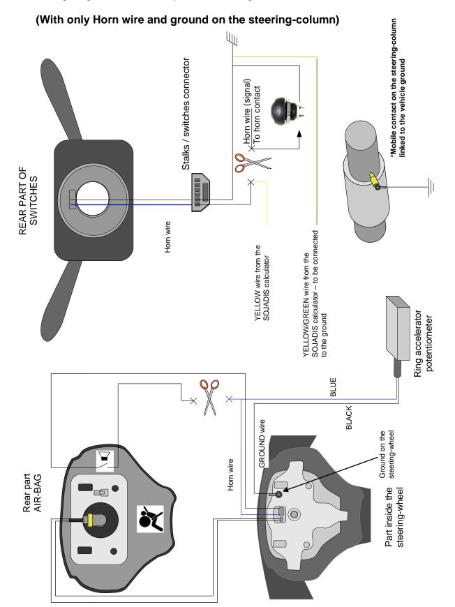
\*The mobile contact to be linked to the ground is not supplied in the kit. Here is the code to order it: cod. HT-ACC-R.13
