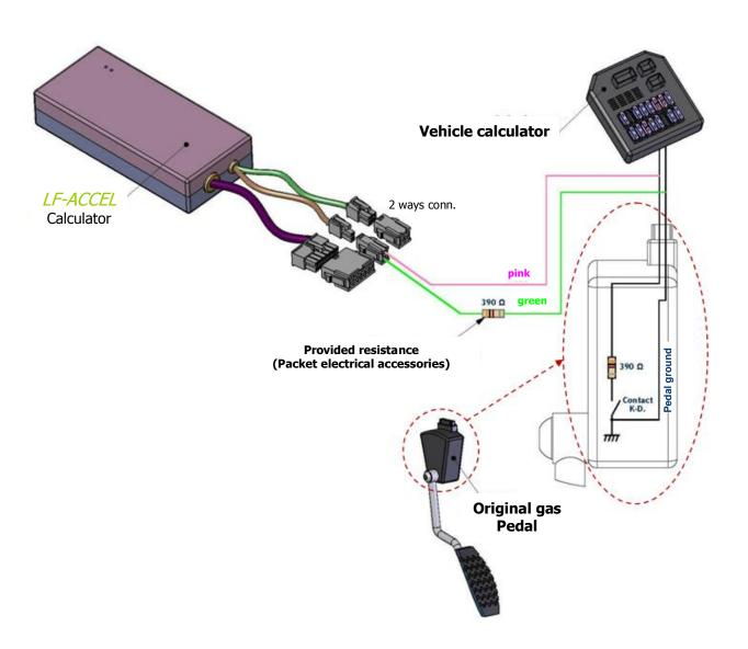
allowing the driver to disable the speed-limiting device if needed.
