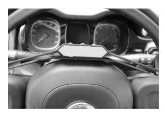
With a Snap-ring / circlip pliers, move the ring support aside (see picture below), in order to lock it against the steering-wheel. Then, tighten both screws.
