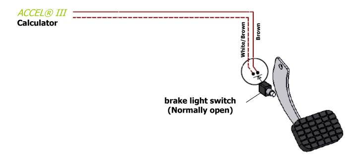
If the vehicle has a normally open brake light switch and has no LED stop lights, wire the 2 brown wires on both sides of the brake light switch.
