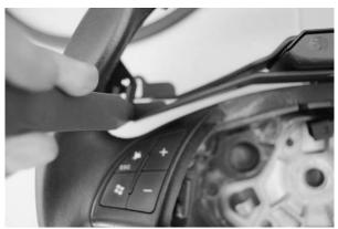
Place the leather-covered ring in the upper part of the sliding support with the "soft" part of the ring towards the driver.
