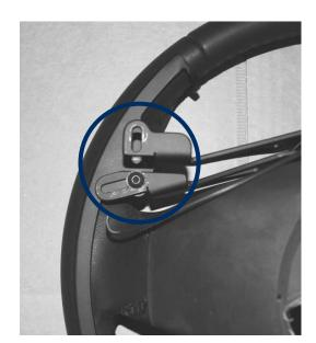
Fix the ring support on a way to not disturb the visibility of the dashboard.
