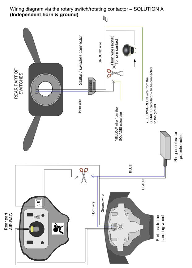
Link the blue wire from the ring accelerator potentiometer to the yellow wire from SOJADIS calculator in option in this diagram. If we cannot use the internal Ground of the steering-wheel, which has a free connection on the airbag spiral, then link the yellow/green wire of the SOJADIS calculator to the black wire of the potentiometer.
