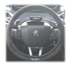
The airbag still works when the ring accelerator is fixed on the steering wheel.
