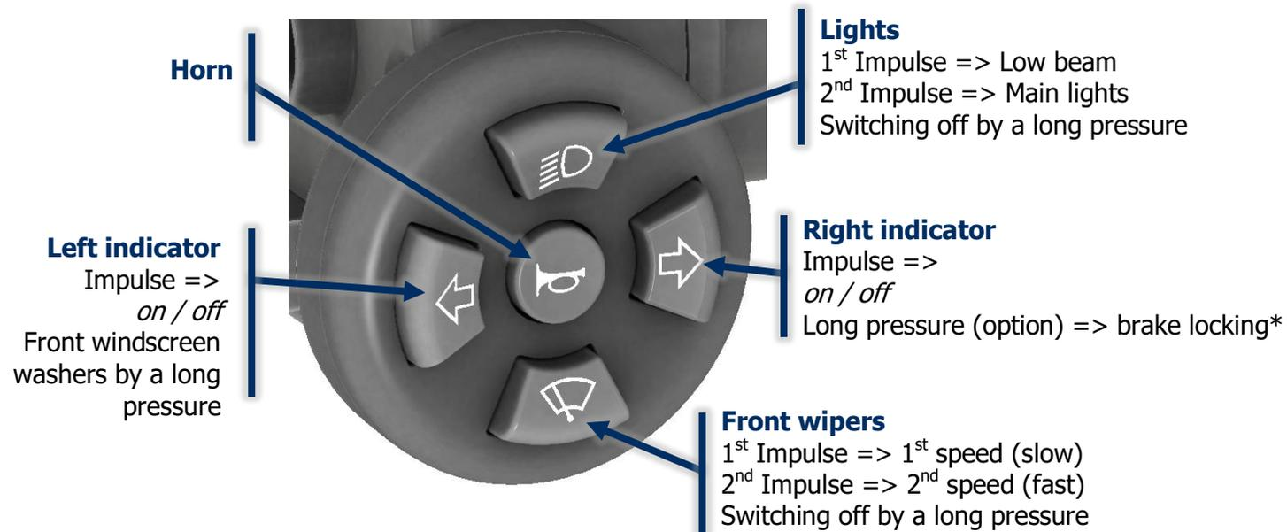
*\*If you have a manual brake Stopdis II FUA with a locking system, you can lock the brake lever by a long press on the right indicator button. Please read carefully the user manual from Stopdis II before using it. SOJADIS Equipement does not assume any liability if an accident or property damage has been occurred due to improper use as described into the manual brake user manual.*
