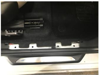
Remove seat front mounting bolts (maybe necessary to loosen rear seat fixing bolts to enable ease of bracket fitting.)
