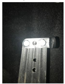
Picture shown of a floor mounted accelerator pedal. For a standard pedal fasten as per brake bracket.
