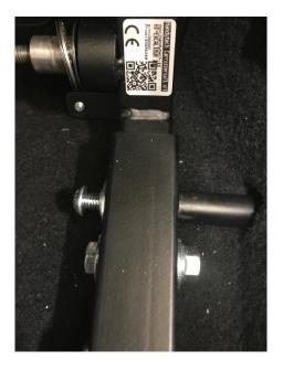
• Tighten seat bracket fixings and rear seat fixings if previously loosened
