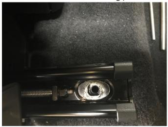
• Slide the Adjustable lever Mounting Bracket over the Lever assembly and place in the footwell. Adjust length to find optimum position for the lever assembly.
