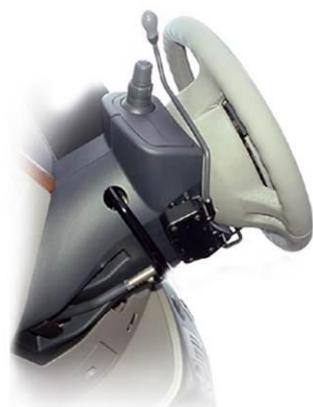
The box mounted under the steering wheel makes possible the conservation of the air-bag.
