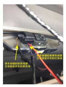
10. Connect our lock adapter to original lock connectors. You can find it behind original latch modular.
