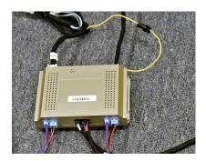
16. Place our control on hatch panel, fix it (ECU) by using a provided screw
