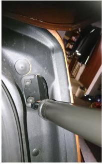
Use original door brackets to install our power strut, cable at this end
