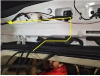
15. Insert all the plugs into the control box (ECU), leave power plug as the last one
