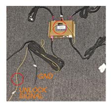
If there is no trunk button in the keyfob, you need to connect our yellow unlock wire to original unlock signal, then you can use remote control - three click unlock button. The unlock signal can be located inside B pillar wire set, that wire has a positive voltage pulse when you click unlock button
