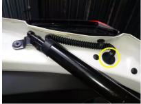
3. Routing strut cable to the latch position
