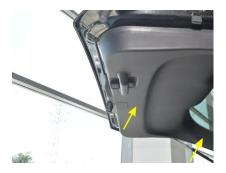
Loosen original gas spring clips by using a screw driver, pull the gas spring out gently. You will need an assist to hold the door when removing the gas springs
