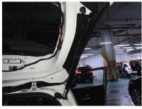
6. Route strut cable through factory hole in door panel
