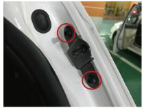
4. Install provided stud & metal washer in top screw hole, use original screw and provided rubber washer to fix in bottom hole
