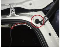
Route strut cable to right side of trunk, where we place control box
