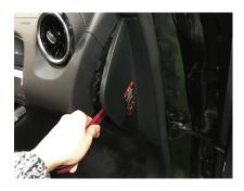
Remove step panel on passenger's side
