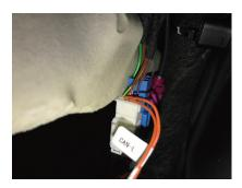
14. Locate original fuse box under passenger's foot mat, insert our fuse plug for power
