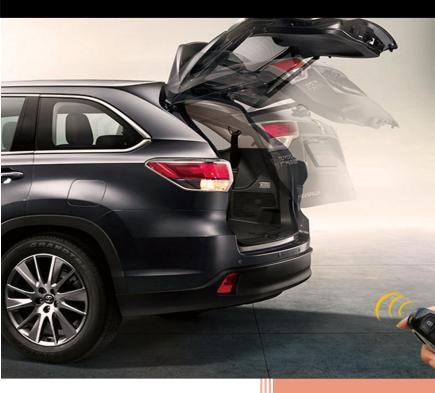
FOR MB GLA This power lift gate kit for MB GLA support automatic trunk open/close control by using 1) original remote control 2) dashboard/front button 3) tailgate/rear button 4) Foot sensor – optional
