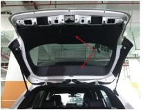
2. Loosen original gas spring clips by using a screw driver, then pull it out. Note you will need assist to hold the door when removing the gas springs
