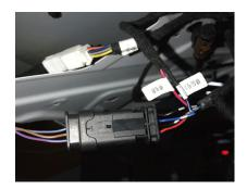
9. Route lock cable and our rear button cable to right side of trunk
