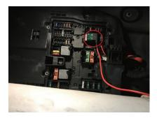
15. Insert all the plugs into the control box (ECU), leave power plug as the last one, you will hear a beep once power connected. Fix control box (ECU) on right trunk, secure by using a provided sticker or string
