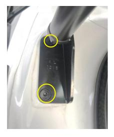
4. Install our power strut, cable at door end
