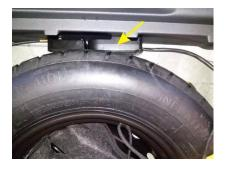
17. Connect all cables to the control unit, leave power cable as the last one, you will hear a beep once power connected
