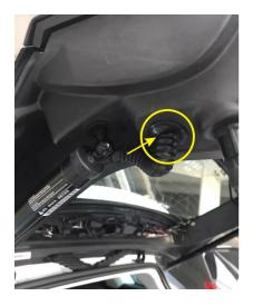
6. Routing strut cable to the lock position (where we place control box)
