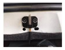
16. Put the latch motor in position and secure it with provided tap.
