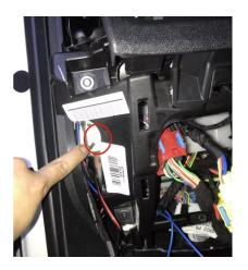
9. Locate original side door connector in B pillar, connect our yellow wire to original white wire for remote control.
