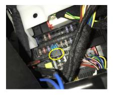
8. Fix our black GND wire to a screw on left side of fuse box
