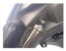
3. Replace original car body bracket to ours, fix with our screws
