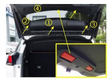
Loosen original gas spring clips by using a screw driver, then pull it out gently. You will need an assist to hold the door when removing the original gas springs
