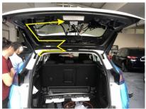
12. Bypass this step if you do not have a foot sensor. Locate OEM trunk switch per picture, connect our foot sensor green wire to original trunk switch signal which is a white wire
