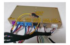
18. Place control box on door panel, secure it by using a provided screw
