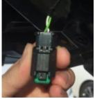
13. Disconnect original lock connector, connect our lock adapter in between
