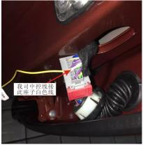
10. Drill a hole in dashboard to install our front button (picture for reference)
