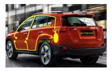
Route rear button cable and lock adapter cable to rear door
