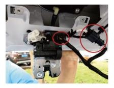
12. Bypass this step if you do not have foot sensor. Connect foot sensor green wire to OEM trunk switch signal
