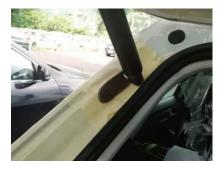
Use original door stud to install power strut, cable at car body end
