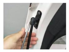
3. Replace original car body brackets to ours, fix with original screws
