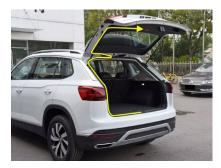
7. Place control box in left side of trunk. Route power cable & CAN-bus cable to driver's dash board
