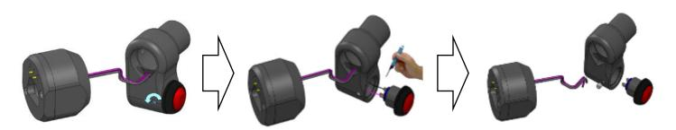
6.2.2 Insert the electrical contact interface into the FUH part.
