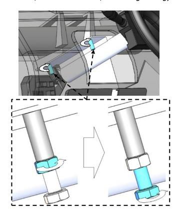
3.2.2 Drill the strut with a drill of 11 mm diameter and a depth of 30 mm.
