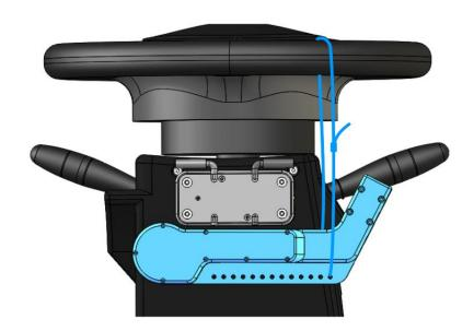
5.2 With a 14mm open-end wrench, turn the pivot axis counter-clockwise (top view) until it stops mechanically. Then tighten both hex-headed screws M6 to a torque of 9.5 N.m.
