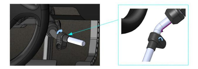
6.2.9 Solder the wires to the button and then insert the button into its holder. Lock the button with the set screw.
