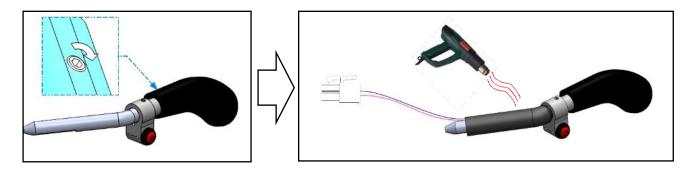
6.1.8 Cut the cover at the indicated length (see below). Please be careful to not cut the harness. Insert a 2<sup>nd</sup> cover all around both wires (about 1 cm length) as indicated below.
