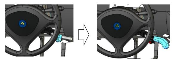
6.1.4 Then adjust the angle of the grip and screw the threated pin M5x8 in order to find the drilling point on the lever.
