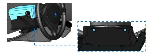
13.3 Reposition the housing below if it has been removed. If necessary, cut the plastic for the secondary rod passing.
