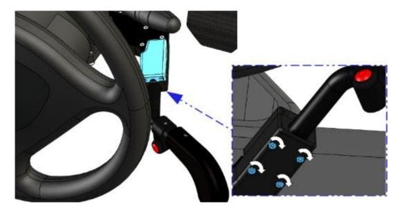
Link to the anchor point positioning
