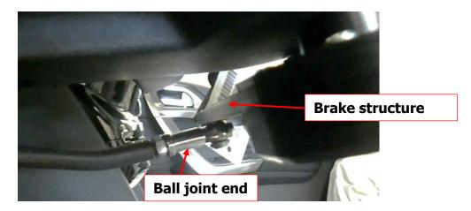
9.3 Shaping the secondary rod FRG according to the part already made (see recommendation in following pages). Use a welding torch to make easier the shaping.
