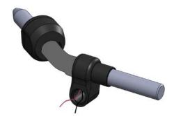
6.2.8 Then adjust the position and inclination of the knob holder, and screw in and tighten the M5x5 set screw.
