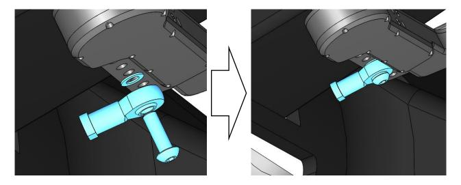
9.2 Use the round part in aluminium (diameter of 6 mm) for defining the shape and the trajectory of the secondary rod (see picture below). We advise you to place the round part in aluminium and **making the braking tests before shaping the rod. For the braking tests, see on page 48 "requirements for braking test".**
