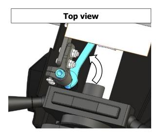
10.2 Then tighten both hex-headed screws M6 to a torque of 9.5 N.m. If you cannot pass a torque wrench, use a 10mm flat wrench.
