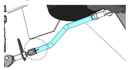
9.6 Remove the secondary rod part and then sold in semi-automatically the FRD part on the secondary rod (soldering MIG). Then, paint the soldered secondary rod.
