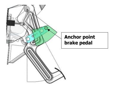
Recommandation for the anchor point positionning under the brake lever structure.
