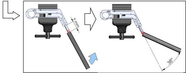
5.7 Heat up the part indicated on the red area at the previous step. Then with the square tube bend at the mark at an angle of about 5° in comparison to the top view (see below)
