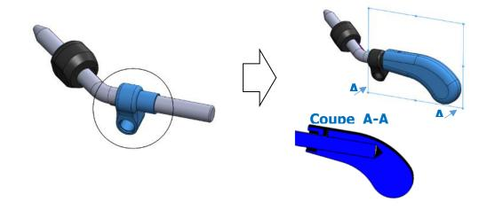
6.2.5 Cut back the FUH part so that the handle is next to the steering wheel.
