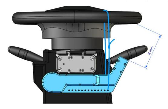
5.4 Si Place the mounting tool STOPDIS II in the vice and insert the FUH part in the mounting tool. Lock the FUH part with the threated pin M8x10.
