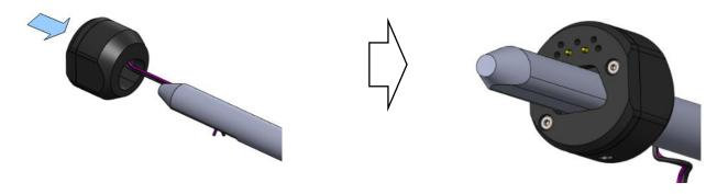
6.2.3 While holding the two plastic parts against the FUH part, slightly tighten the threaded pins on the bottom.
