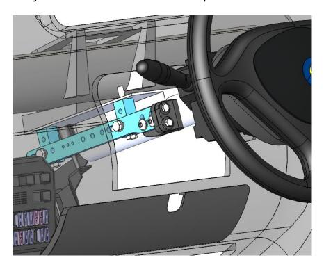
3.1.3 Adjust the adjustable sleeve so as the socket axis is closed to an angle of 90° to the casing under steering wheel when it is installed (screw the casing under steering-wheel if necessary).
