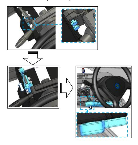
To remove the socket you can also use an M5 screw (tighten the M5 screw to remove the socket). Please remove this screw after positioning the brake lever.
