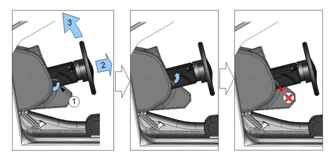
2.2 Remove the flywheel housing – under part; over part if possible (see examples below).
