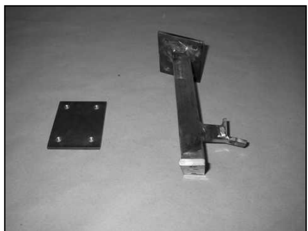
Picture 11 (bracket with counter-plate)
