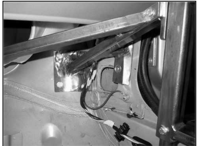
Picture 17 (tie-rod upper mounting)
