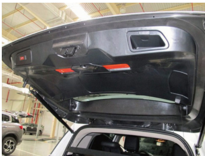
16. Initialize system after installation - manually lift rear door to desired height ( must be 10mm less than max height ), keep on pressing our rear button 3 seconds until a beep is heard, short press our rear button to close door, when the door is fully closed with a beep, it means the system is initialized and ready for use.
