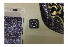
10. Locate original UNLOCK connector inside B pillar, connect our yellow wire to original unlock signal for remote control.
