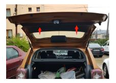
2. Loosen original gas spring clips by using a screw driver, pull the gas spring out gently. You may need assist to hold the door when removing the original gas spring
