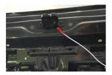
13. Insert all plugs to the control unit, leave power cable as the last one, our rear button has backlight once power connected.
