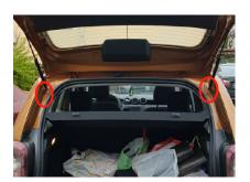
4. Replace original door stud & washer to ours. Install our power strut, cable end at door, drill a hole in door panel to route strut cable
