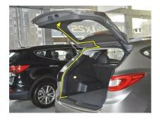
12. Locate lock connector behind original latch, disconnect it and re-connect with our lock adapter in between
