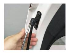
3. Remove original car body stud & washer, install our bracket, fix with our screws
