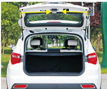
6. Remove original trunk panels
