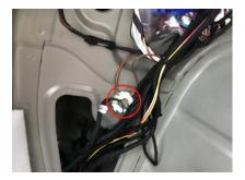
8. Locate original lock plug behind original latch, connect our blue lock wire to original pin 6; cut original pin 5 off, connect our orange wire to latch end, connect our red wire to another end
