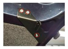
Install power struts, cable end at trunk
