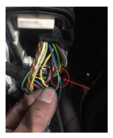
12. Insert all the plugs into the control box (ECU), leave power plug as the last one. Place our control on hatch panel, fix it (ECU) with sticker or string tightly
