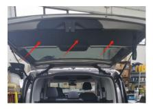
Loosen original trunk panels on both sides
