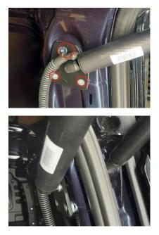
4. Install our door brackets on both sides, fix with provided rivet nuts. Note you will need to drill three diameter 9mm holes to fix nuts
