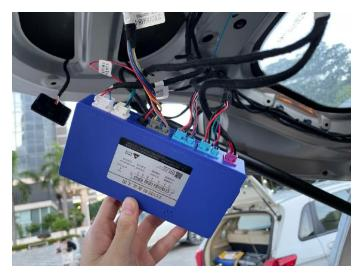
13. Drill a hole to install our rear button. Restore hatch panel, installation completed
