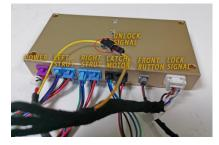
Put the control box in rear door panel, secure with provided screw
