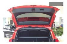
2. Loosen original gas spring clips by using a screw driver, pull the gas spring out gently. You need an assistance to hold the door when removing the gas springs, the door is very heavy
