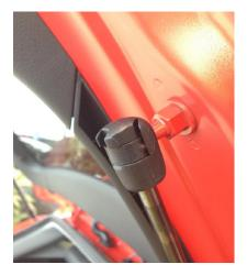
Original car body bracket is welded on the car, it cannot afford our power strut force thus we provided extra brackets to reinforce it per the following steps
