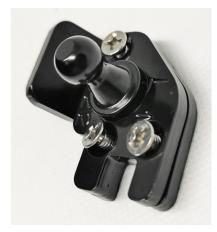
4. Install our power struts, cable at car body end. <u>MUST</u> INSTALL TO THE BALL STUD FROM OUR BRACKET, NOT ORIGINAL BRACKET
