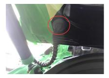
Routing strut cable to the lock position (where we place control box)
