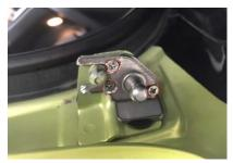
Attach our bracket support to original car body bracket, secure with our M8 screw & nut (x1)
