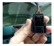
15. Insert all the plugs into the control box (ECU), leave power plug as the last one, you will hear a beep once power supplied
