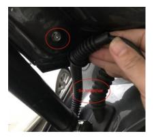
5. Replace original tailgate latch to our power latch, fix with original screws
