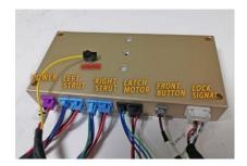
11. Place control box (ECU) on tailgate panel, fix it by using a provided screw
