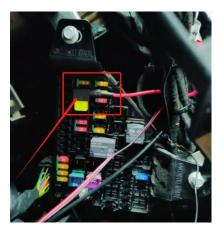
Fix our GND wire to screw on right side of fuse box
