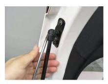
3. Replace original car body brackets to ours, fix with our screws, use original door stud to install power strut
