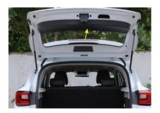
2. Loosen original gas strut clips by using a slotted screwdriver, then pull gas struts out gently. Be aware factory door panel is very heavy, use an assistance to hold the door when removing both gas struts
