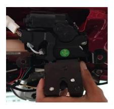
6. Connect original lock plug to our lock assemble (harness)
