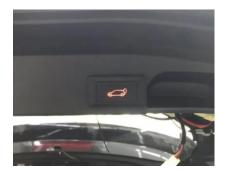
10. Insert all the plugs into control box (ECU), leave power cable as the last one, or short press our rear button to activate system if you do not see backlight on it
