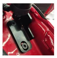
4. Install our power struts, cable end at trunk, route strut cable through factory reversed holes in door panel
