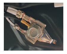
12. Disconnect original lock connector, re-connect with our lock adapter in between
