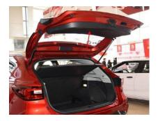
2. Loosen original gas strut clips by using a slotted screw driver, pull the struts out gently. You will need an assist to hold the door when removing these factory struts
