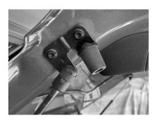
4. Replace original car body brackets to ours, fix with our M6 screws
