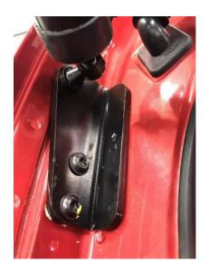
5. Install power struts with cable end at car body, route strut cable through factory reversed holes in door panel
