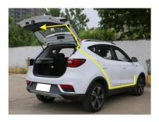
11. Fix our GND to a factory ground screw in rear door panel tightly, make sure that screw has no paint on surface for good power flow
