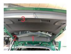
2. Loosen original gas strut clips by using a slotted screwdriver, then pull gas struts out gently. Be aware factory door panel is very heavy, use an assistance to hold the door when removing both gas struts
