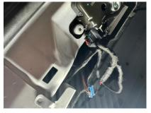
Put our latch motor in left side of trunk, make sure to route latch string smoothly, do NOT curve too much on both ends
