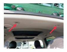
6. Route power cable to engine hood, route front/dash button to driver's dashboard, route rear button cable to rear door
