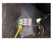
8. Locate original battery in engine hood, fix power cable to battery positive screw
