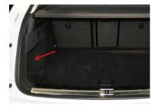
Fix latch motor with provided nut and screws on left trunk panel tightly
