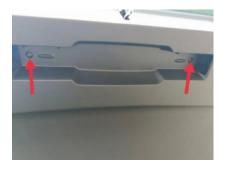
Remove original rear door panel with a removal tool per sequence number
