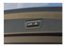
12. Bypass this step if you already has a factory trunk button in dash, which can release original door latch (not unlock), you can use original trunk button. Otherwise drill a hole to install our dash button
