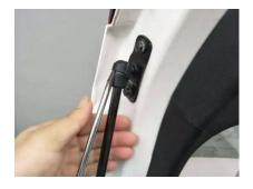
3. Use original door bracket and trunk stud to install power struts, cable end at door. Note install strut with one plug on left, strut with two plugs on the right side
