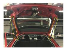
4. Replace original trunk stud to our bracket, fix with our M8 screws
