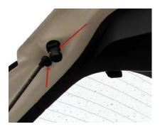
Attach small metal fitting plate to our door plate with a M6 screw, route it through original rubber block hole, do not fasten screw until bracket is placed properly
