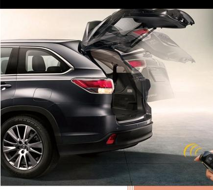
For Nissan Qashqai This power lift gate kit for Nissan Qashqai support automatic trunk open/close control by using 1) original remote control 2) dashboard/front button 3) tailgate/rear button 4) Foot sensor – optional
