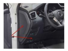
Locate fuse box on left side of das. Remove original 20A fuse, insert it to our power plug, finally insert our fuse power plug back to the original socket
