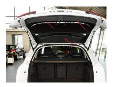
3. Loosen original gas spring clips by using a slotted screwdriver, then pull gas struts out gently. Be aware factory door panel is very heavy, use some assistance to hold the door when removing gas struts
