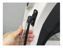
3. Use original door stud and trunk bracket to install our power strut, strut cable at trunk end
