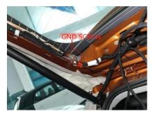
8. Connect our lock assembly harness to original lock plug
