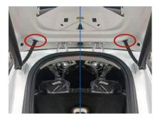
Routing strut cable to rear door
