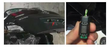
12. Disconnect original lock plugs, re-connect with our lock adapter in between
