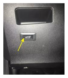
11. Bypass this step if you do not have foot sensor. Connect our foot sensor green wire to original trunk switch signal which is white wire
