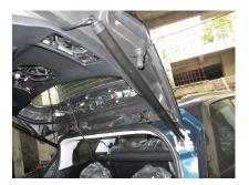
Cut a slot on door panel to route strut cable through per arrow
