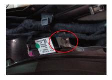
10. Drill a hole in dashboard to install our front button, picture for reference only
