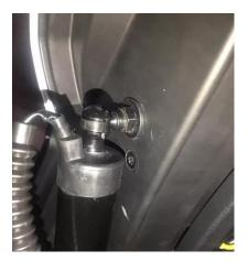
4. Replace original car body brackets to ours, fix with original screws
