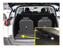
8. Routing striker motor cable to rear door, route power cable to driver's dash
