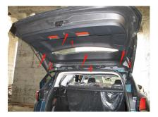
2. Loosen original gas spring clips by using a screw driver, pull the gas spring out gently. You will need an assist to hold the door when removing the gas springs
