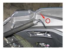
Routing strut cable to rear door
