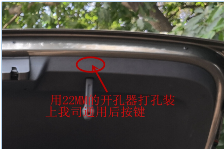
13. Drill a hole in door panel and install our rear button
