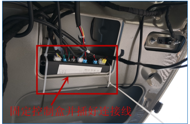
12. Insert all plugs in control box, put control box on door panel and secure with sticker
