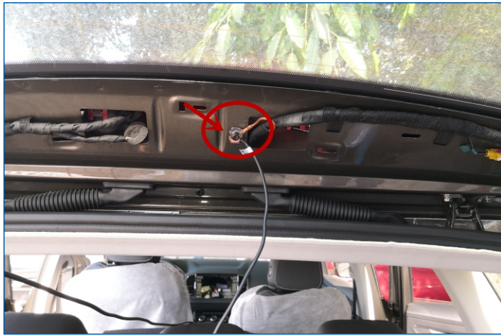
11. Ground our GND wire to a screw in door panel
