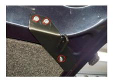
Install power struts, cable end at trunk
