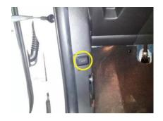
10. Locate original unlock signal inside A pillar
