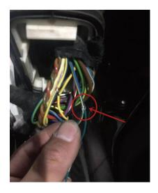
11. Insert all the plugs into the control box (ECU), leave power plug as the last one. Place our control on hatch panel, fix it (ECU) with sticker or string tightly
