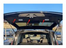
Loosen original trunk panels on both sides
