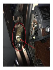
Connect our green wire to original yellow/blue wire for remote control(3x unlock button). Contact Autoease for support in case your wiring set does not look the same as picture
