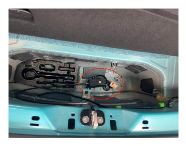
7. Disconnect original latch/lock connector, re-connect with our lock adapter in between
