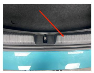
2. Loosen original gas spring clips by using a screwdriver, pull the gas spring out gently. You will need an assist to hold the door when removing the gas springs
