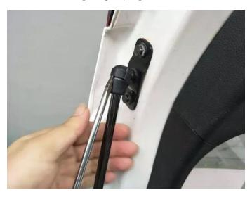
3. Remove the original door studs & washer, replace to our short studs and washers.
