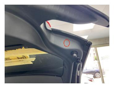
6. Replace original latch striker to ours, fix with provided screws
