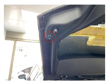
Remove the original trunk studs & washer, replace to our long studs and washers.
