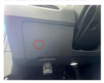
14. Drill a Ø20mm hole to install our rear button
