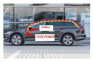
10. Pry panels under driver's dash to access fuse box, pry panels under steering wheel off to access CAN-bus signal
