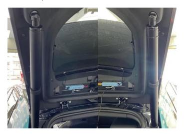
\*\*\* NOTE cable end at door. Check strut ball joint are pushed into position once struts are installed, make sure ball joint clip is flush on surface. Manually lift the door up and down to make sure there is no interfere when closing.
