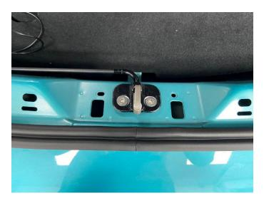
Place latch striker motor inside of trunk
