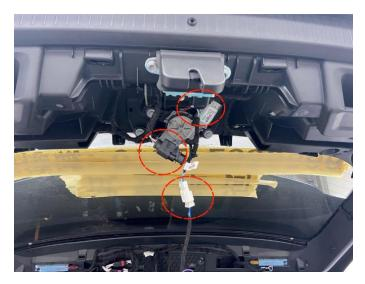
8. Ground our GND wire to a screw in right side of trunk. Make sure that screw has no paint on surface for good conductivity
