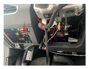
11. Locate original fuse box, remove original 30A fuse, insert it back to our fuse plug port, finally insert our fuse plug to original fuse port
