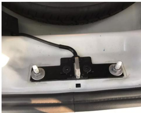
Place latch striker motor in left side of trunk
