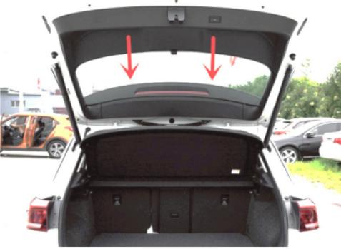
2. Loosen original gas spring clips by using a screw driver, then pull it out gently. Note you need a help to hold rear door when removing the original gas spring
