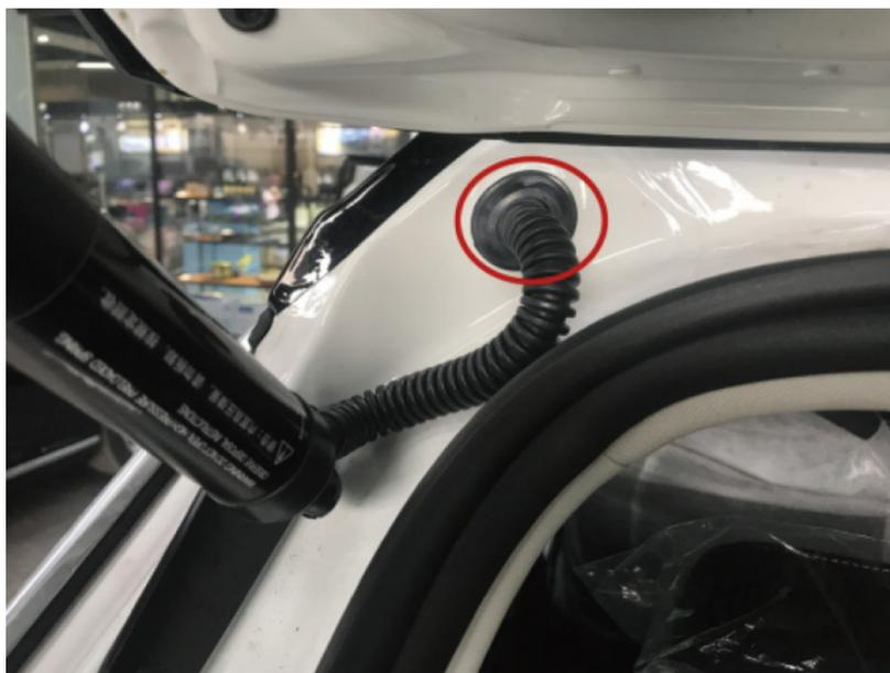
5. Remove trunk panel, use our latch striker to replace original one, fix with original screws
