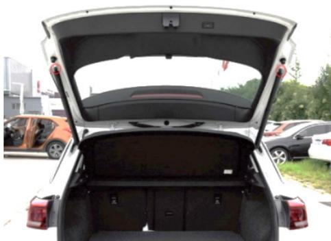
4. Use factory reserved hole in left trunk body to route strut cable, drill a hole at right side to route cable
