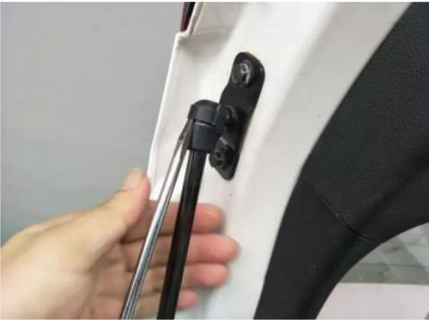
3. Replace original car body brackets to ours, fix with original screws
