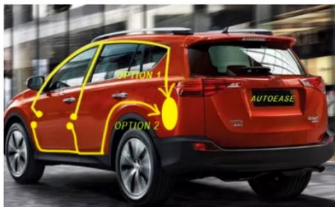
Route rear button cable and lock adapter cable to rear door
