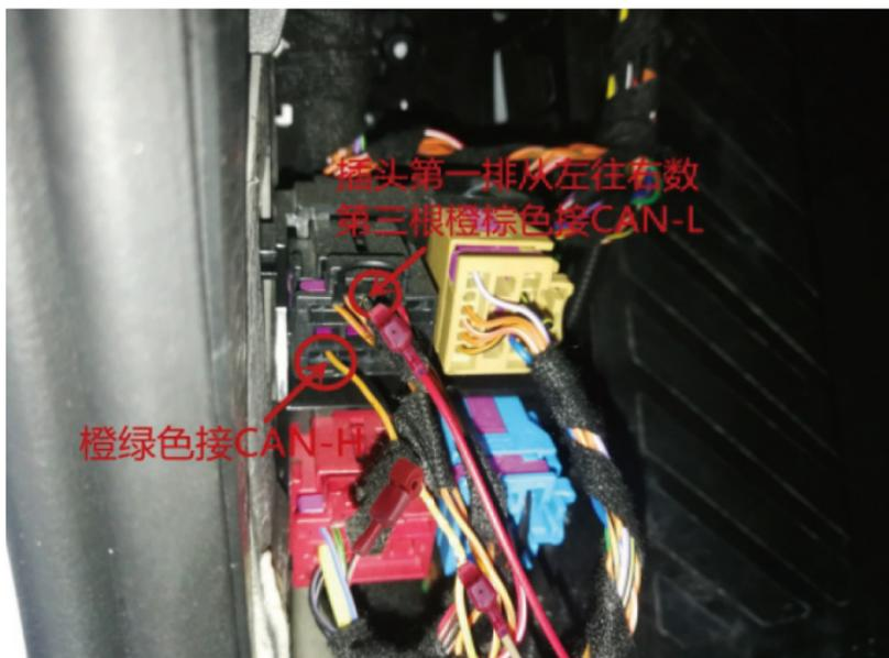
11. Connect our lock adapter in between original lock connectors
