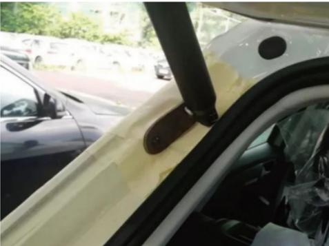
Use original door stud to install power strut, cable at car body end
