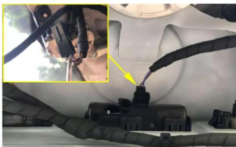
13. Insert all the plugs into control box (ECU), leave power cable as the last one, you will hear a beep once power connected. Fix the control box (ECU) to left side of trunk by using a sticker or strings
