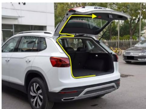
7. Place control box in left side of trunk. Route power cable & CAN-bus cable to driver's dash board
