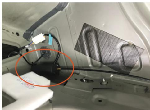
6. Routing power striker cable to rear door panel
