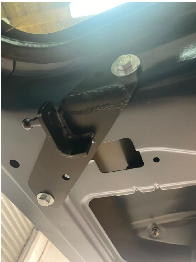
Install power struts, cable end at trunk
