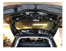
2. Loosen the original gas spring clips by using a screw driver, then pull it out. Note you may need help to hold the gate when removing the original gas spring
