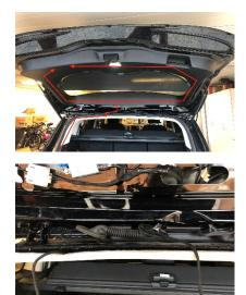
6. Remove a support like picture so you can access the original latch
