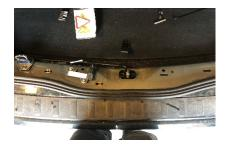
5. Route \*power cable, \*front button wire to rear door (control box position)
