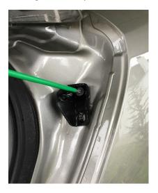
Remove original door bracket screw per picture, install our ball stud and washers in the screw hole then install our strut, cable at this end
