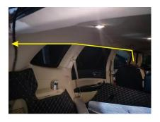
Route \*power cable \*front button \*latch motor cable to control box position
