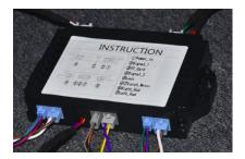
Secure the control box (ECU) on hatch panel by using a provided 3M tape
