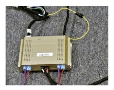
16. Place control box(ECU) inside hatch panel, secure it by using a provided screw
