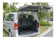
Loose the original gas spring clips by using a screw driver, then pull it out. Note you may need help to hold the gate when removing the original gas spring
