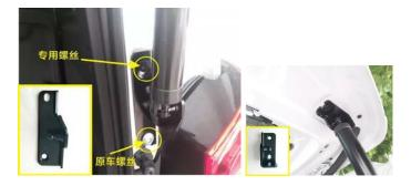
5. Remove two screws of taillight, then loosing the light. Routing pole cable through the gaps as below picture.
