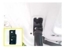
3. Replace original bottom left bracket with our bracket, fix with provided screws. Note stud headed inward.
