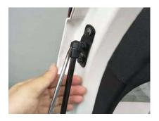
2. Replace original top left bracket with our bracket, fix with provided screws. Note stud headed outward.
